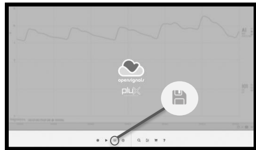
Fig. 4. Signal Storage Operation
