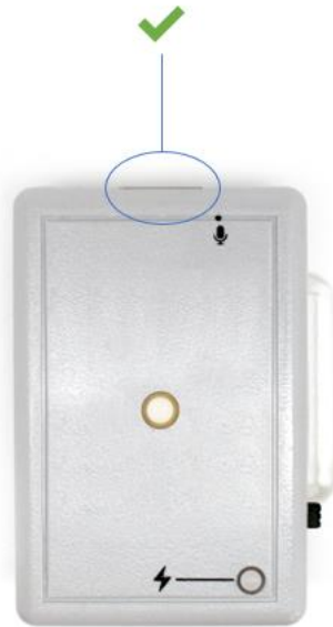
Figure 7: Connect the EGG to the analog input channel of the biosignalsplux Solo (openBAN).
