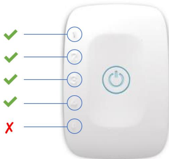
Figure 5: EGG compatible biosignalsplux channels (green checkmarks).
